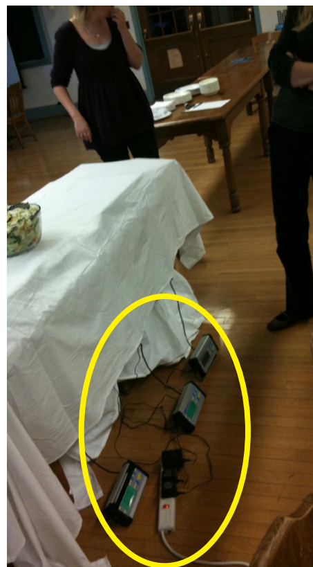
To help prevent the fasters from being too self-conscious about what and how much they ate, we have scales under the table cloth. They are read off the three monitors on the floor.
